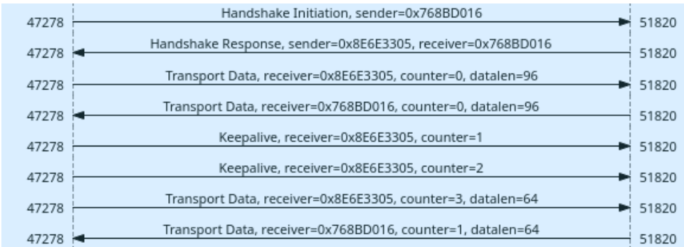
Figure 6.2: Flow graph between two WireGuard peers as seen in Wireshark
